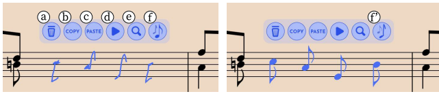
Figure 4: A note selection and the associated contextual menu: a) erase selection, b-c) copy-&-paste selection, d) play back selection, e) find occurrences of the selection, f/f') switch between engraved and handwritten representations.
